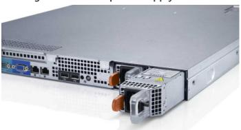
The PowerEdge R320 supports up to two AC with 1+1 redundancy, auto-sensing, and auto-switching capability.
